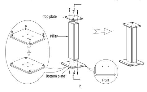
B. Place speaker on stand, making sure the holes on bottom of speaker align with the 4 holes on the top plate.
