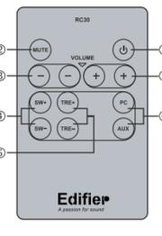
**Note:** "SW +/-" and "TRE +/-" are trimmer adjustments which are both tone controls based on master volume level. "SW +/-" ranges from -9 to +9; "TRE +/-" ranges from -7 to +7; minus figure refers to attenuation, positive for boost, and "0" for no boost and no attenuation. 3 seconds no action in trimmer mode, the system will return to master volume adjustment.
