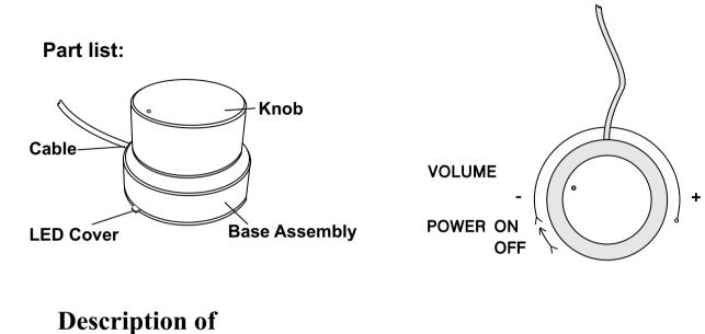
In addition to using the volume control on the back panel, there is a specially designed line level control for the S2000V to control power and volume.
